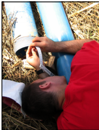
Measuring the Thickness of a PVC Casing Pipe | Photo D. Saulnier
